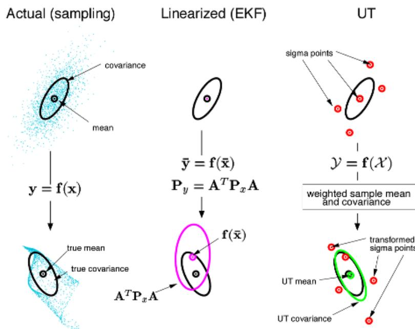
Figure 35: An overview of Unscented Kalman Filter (UKF)
