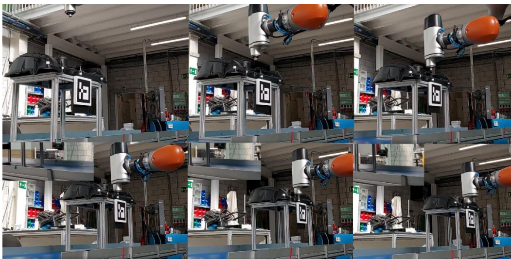
Figure 32: First demonstration of successful screwing in motion
