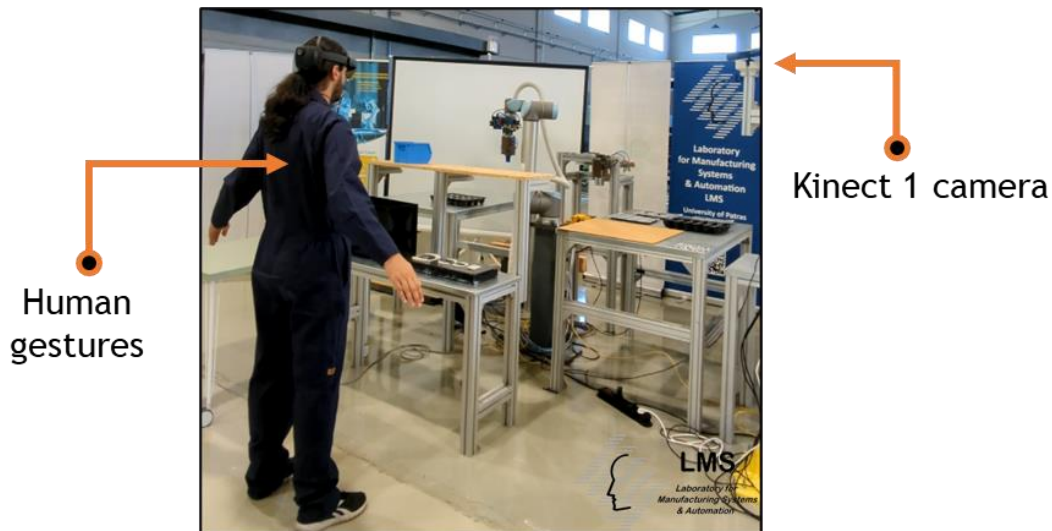
Figure 71: UR10 controlling through the human gesture recognition module
