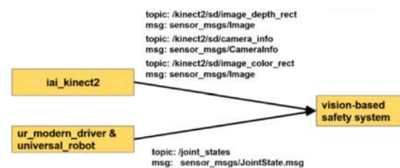
Figure 5 Data streams connected to Vision Safety system node
