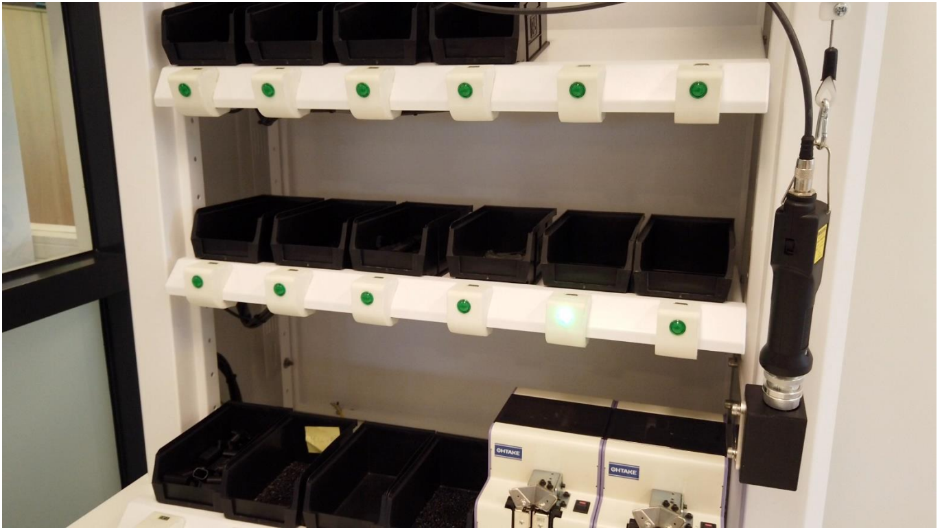
Overview of pick-2-light production cell with manufacturing bins, LED indicator and proximity sensors.
