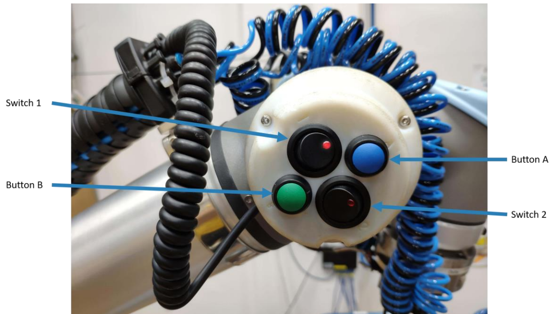
Figure 2: The button interface used for manual guidance. The button interface replaces one of the standard UR-10 joint covers. The button states are connected through the robot controller I/Os.
