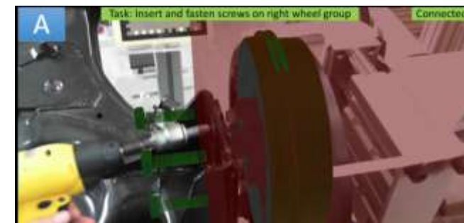
AR based application – Operator's field of view
