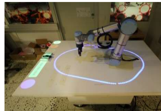
Projection-based safety zone around robot
