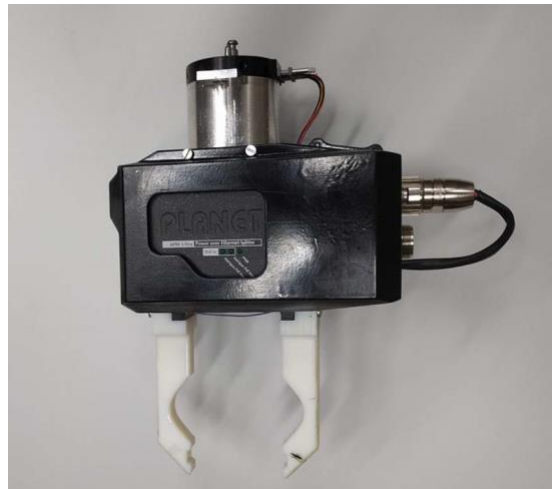
Figure 2: The ROS peripheral interface attached to a robot servo gripper.
