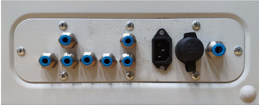
Figure 4: Example of inputs and outputs to the enclosure of the ROS peripheral interface.
